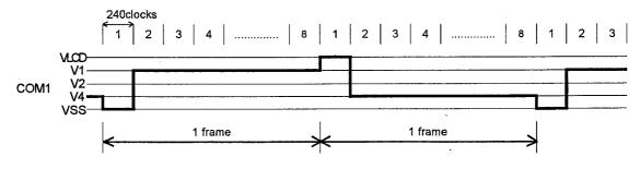
1 frame = 6.54(us) x 240 x 8 = 12.55(ms) Frame frequency = 1 / 12.55(ms) = 79.68(Hz)
