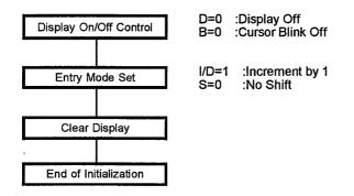
Note : If the condition of power supply rise time described in the Electrical Characteristics is not satisfied, the internal Power On Initialization Circuits will not operated and initialization will not performed. In this case the initialization by MPU software is required.
