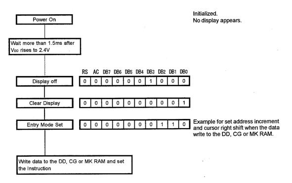
Note : When the Icon display function using, the system should be initialized by software initialization.
